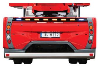
/ The newly designed vehicle rear combines function with warning elements. Protected by a transparent cover, a strip of warning lights extends across the entire rear width to secure both the vehicle as well as the LED floodlights.
