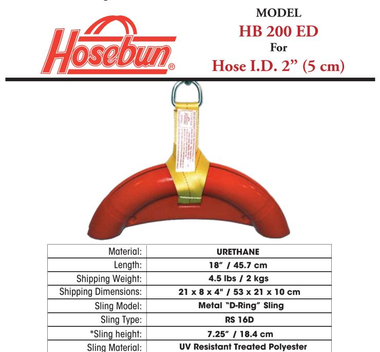
Notes: Also available with Type 4 Hook-Eye sling (Model # RS 234H) for heavy duty jobs. (WLL for RS 234H: 2000lb / 907kgs @ 5:1 or 648kgs / 1428lbs @ 7:1)
