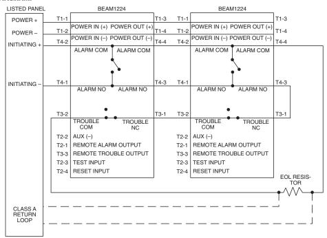
NOTE: If other sensors are installed on the same loop, a listed end of line power supervision module is required.
