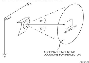
FIGURE 5B. REFLECTOR MOUNTING GUIDELINES
