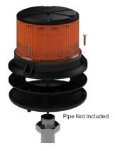
Using the hardware provided, secure the beacon to the pipe-mount adapter, feeding the wire down through the center of adapter plate. After making the appropriate wiring connections, feed the wire through the pipe and tighten the beacon onto the pipe. Tighten the adjustment nut to complete the installation.
