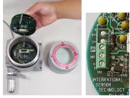
Figure 1 – Remove transmitter cover and pull upper circuit cards straight upward. TB2 is on the left side.
