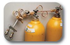
An **air cylinder pressure regulator** is a required accessory when air-line respirators operate from a cylinder. This dual-gauge regulator receives the varying outlet pressure from the cylinder, reduces it, and regulates it to a constant pressure of approximately 80 psig, the optimum pressure for operation of the regulator.
