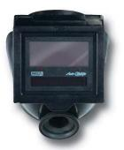
**Welder's adapters** are used for eye protection in welding applications where respiratory protection is required, and are easily installed over a lens. Clip-on style adapter can be easily removed, whereas the integral adapter model is used in place of the facepiece lens. Both models are made of polycarbonate and feature a flip-up lens with large 4-1/2" x 5-1/4" (11.4 cm x 13.3 cm) vision area.
