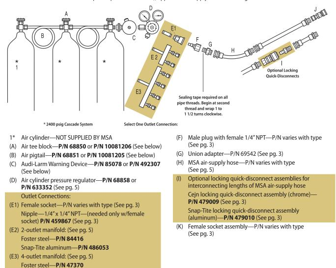
**Tee blocks and pigtails** are used to connect a bank of cylinders together, extending your air supply. The coupler tees, which make a connection between the supply cylinder valve and the pigtail, and the outlet connection, are constructed of brass, while the pigtails, joining the supply cylinders, are made of tubular copper or stainless steel braided hose.
