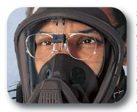
**Spectacle kits**, used by workers who must wear corrective lenses, are easily inserted into Ultra Elite or Advantage 4000 Facepieces. Kits includes wire support, rubber guide, and one pair of metal frame spectacles. One size of spectacle frame is used (S-7 shape, 44-mm lens size) with universal bridge corrective lenses that can be obtained from local sources. The spectacle kit may be worn in conjunction with a nosecup.
